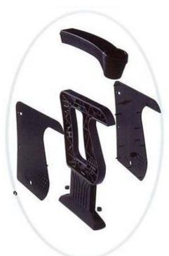
The seat-tipping mechanism is housed in the side panels manufactured by injection using technical materials which carry the seats' tipping axes, equipped with a safety bridge which prevents them accidentally popping out. The bearings are attached to the side panels by steel blued DIN 916 M6 screws.
