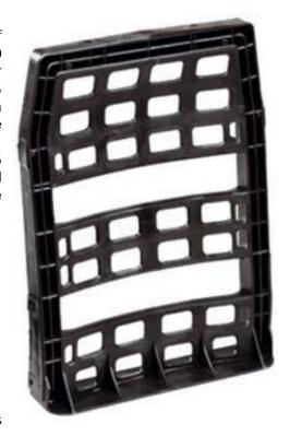
The back of the backrest is protected by a reinforced 5 mm.-thick outer back over the whole surface and 10 mm. in the structural support sections, made by high-impact, black, polypropylene copolymer injection, which is what strengthens the seat via 2 DIN 603/555 M7 70 mm. fixing screws on each side and non-slip washers, in turn fixed to the structure via 4 black, zinc-coated, 7 x 65 TORX screws.
